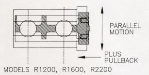
The chucks are effectively sealed to prevent chips and coolant from entering and causing excessive wear to the working mechanism. Self-centering chucks are capable of repetitive accuracy to .001" T.I.R. as standards and as good as .0005" T.I.R. on certain applications. All models come with flat backs requiring an intermediate mounting plate for most machines.
